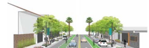
D A Street (Diodora Ave to 3rd St): New bike lanes (either colored green or shown or simply striped with white paint) along with new street trees or existing empty tree planters, new pedestrian-scale street lights, and new red brick crosswalk with curb extensions and palm trees to mark the crossing. Such improvements could surely be made in phases, as funding allows.
