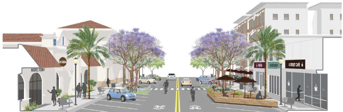
b A Street (3rd St to 7th St): Back-in angled parking, landscape enhancements at mid-block crosswalks, bike corrals, and parklets can all add life to A Street's retail environment.
