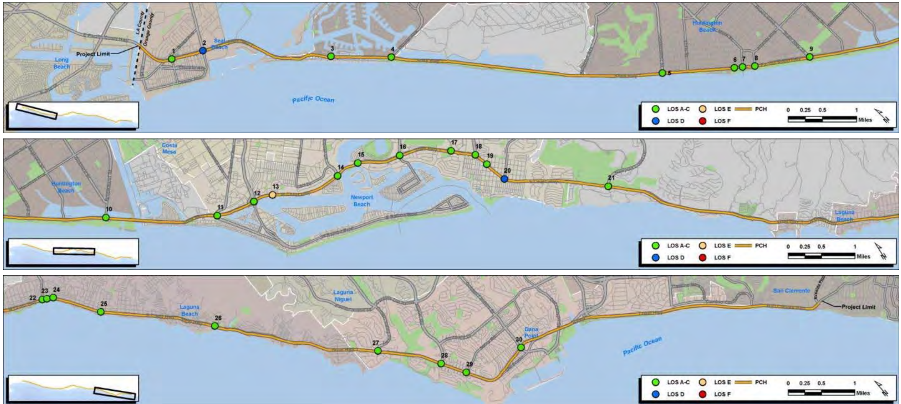
Figure 2.11: Existing PM Peak Hour ICU LOS
