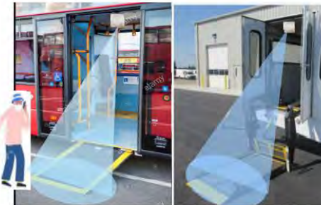
Lbeacon with radiation beam outlining the opened door and boarding ramp
