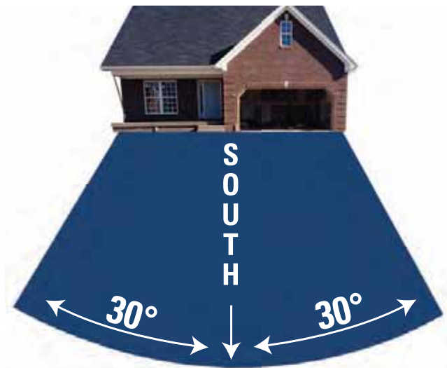
FIGURE 5.3 Orienting Buildings for Best Solar Access
